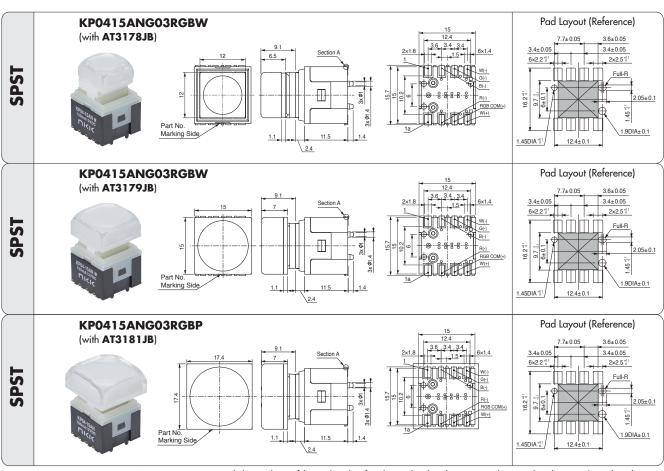
🖂 Area comes into contact with the metal part of the product, therefore this needs to be taken into consideration when designing the PC board pattern.
