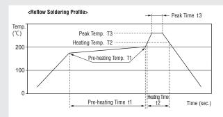
Set the configuration of the reflow furnace so that the product terminal temperatures meet the pre-heating and heating temperatures in the reflow soldering profile conditions (T1 and T2). Make sure the product temperature does not exceed the peak temperature (T3).
