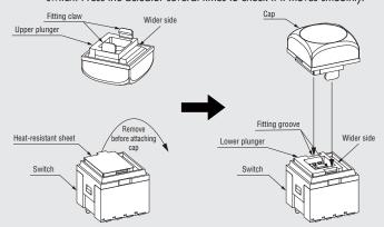
When operating the switch, make sure that an actuator is securely attached. Please note that operating the switch without an actuator or with an actuator mounted incompletely may cause a malfunction or other problems.
