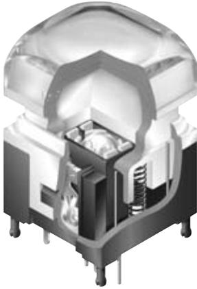
Miniature audio/video pushbutton incorporates a metallic pin rail that accentuates silent, smooth operation. Unique actuation guide provides indications of circuit transfer. Tactile, nontactile, or tactile/audible choices. Superb switching resistance exceeds 5 million operations. Compact size with longer stroke options of 4.5mm for KP01, or 3.5mm for KP02. Light operability with an operating force of 1.6N.
