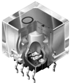
Subminiature, smooth-operation pushbutton, soft touch actuation achieved by mechanical silicon rubber structure. Entire cap is fully illuminated. Both standard (1.5N ±0.5N) or high (2.5N ±0.8N) operating force options. Compact design of only 12.5mm from PC board to top of cap.
