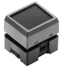
IS15BBFP4RGB RGB LED Option and Black and White LCD Mode
