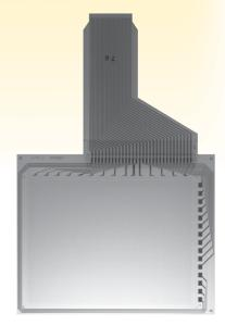
FT Series Touchscreens will be produced with a new ANR (Anti Newton Ring) film to support high resolution LCD monitors.
