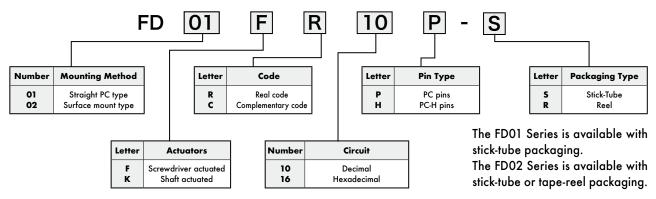
▶The Shaft actuated type is only available for models with "Real code" and "PC pins."
