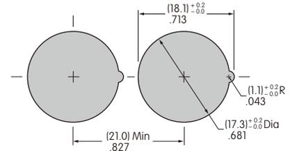
Allow .827" (21.0mm) distance from center-to-center between switches when mounted side-by-side.
