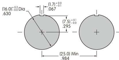
Allow .984" (25.0mm) distance from center-to-center between switches when mounted side-by-side.
